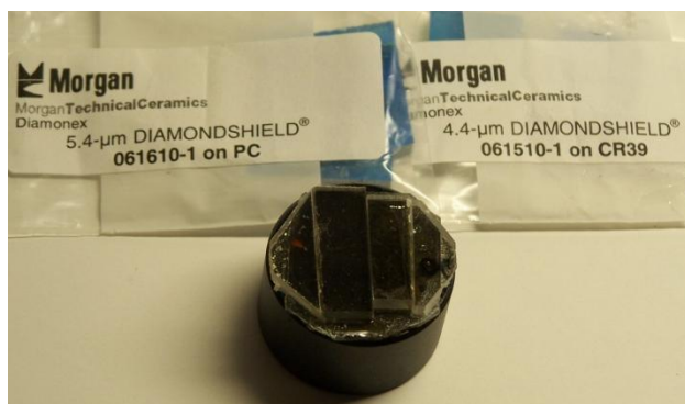
Figure 1: Four diced wafer samples mounted on a sample puck ready for testing.
